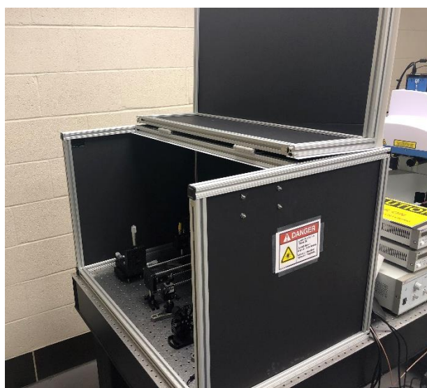
Figure 2.1: Light-proof enclosure for optical components.
