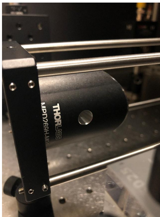
Figure 2.12: Off-axis parabolic mirror with centered hole for alignment beam.
